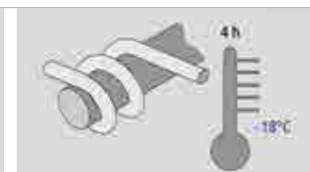
Flexibilitäts-Test CSA-C 22,2, Nr. 227, 3-M91 Flexibility test CSA-C 22,2, No. 227, 3-M91
